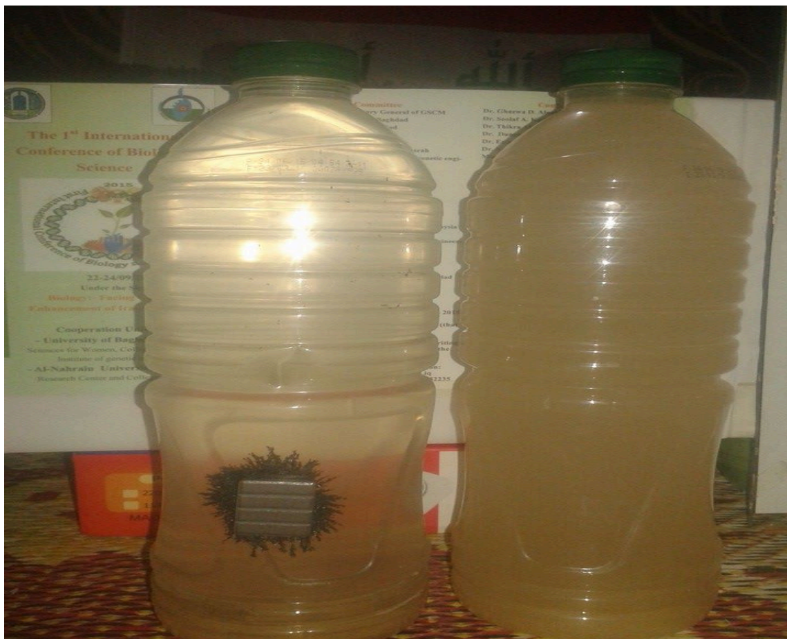
Figure 7. The separation of Magnetite iron Oxide Nanoparticles from water by Magnetic bar.
