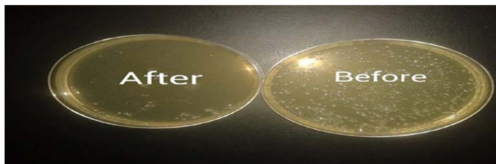
Figure 6. Antibacterial effect of magnetite iron oxide nanoparticles against Escherichia coli polluted water.
